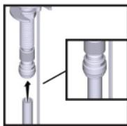
**STEP 3** – Push end of gray outlet tube into adapter connection until it stops (approximately 3/4").
