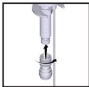
**STEP 2** – Thread on adapter fitting to the shank.
