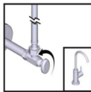
**STEP 4** – Turn water on. Check for leaks. Installation complete.
